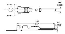
Tab contacts are manufactured from 0.2 [.008] thick material
