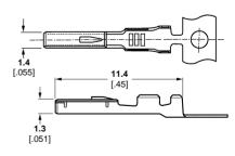
Receptacle contacts are manufactured from 0.2 [.008] thick material.
