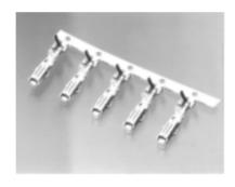
Receptacle contacts are manufactured from 0.3 mm [.012 in.] thick material. Uncrimped contact length is 16.5 mm [.650 in.]
