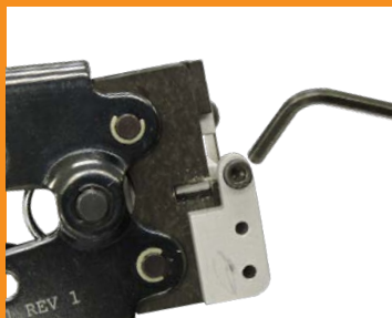
Adjust terminal stop screw to position tab with cutting shear
