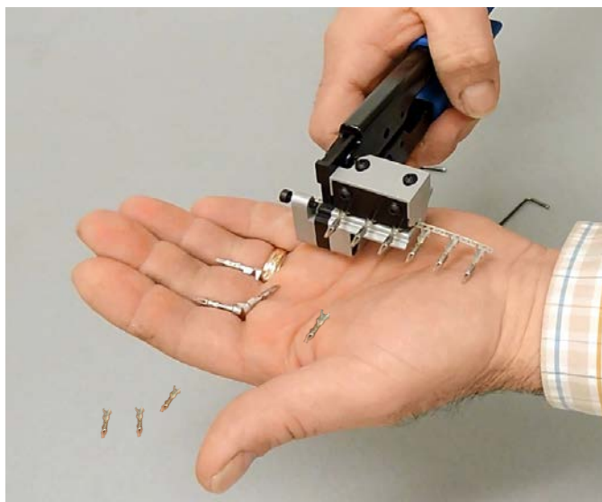
Adjust terminal stop screw to position tab with cutting shear
