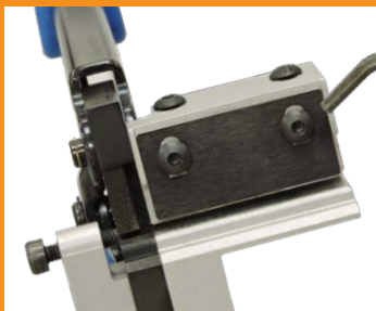
Adjust height with the black adjustable plate using vertical screws
