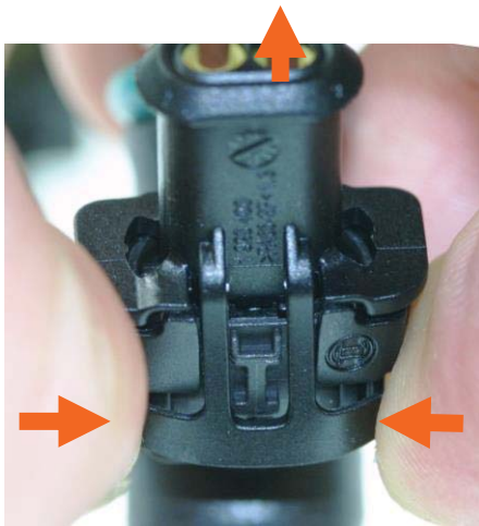
Figure 7: Disengagement the locking element from the locking notch
